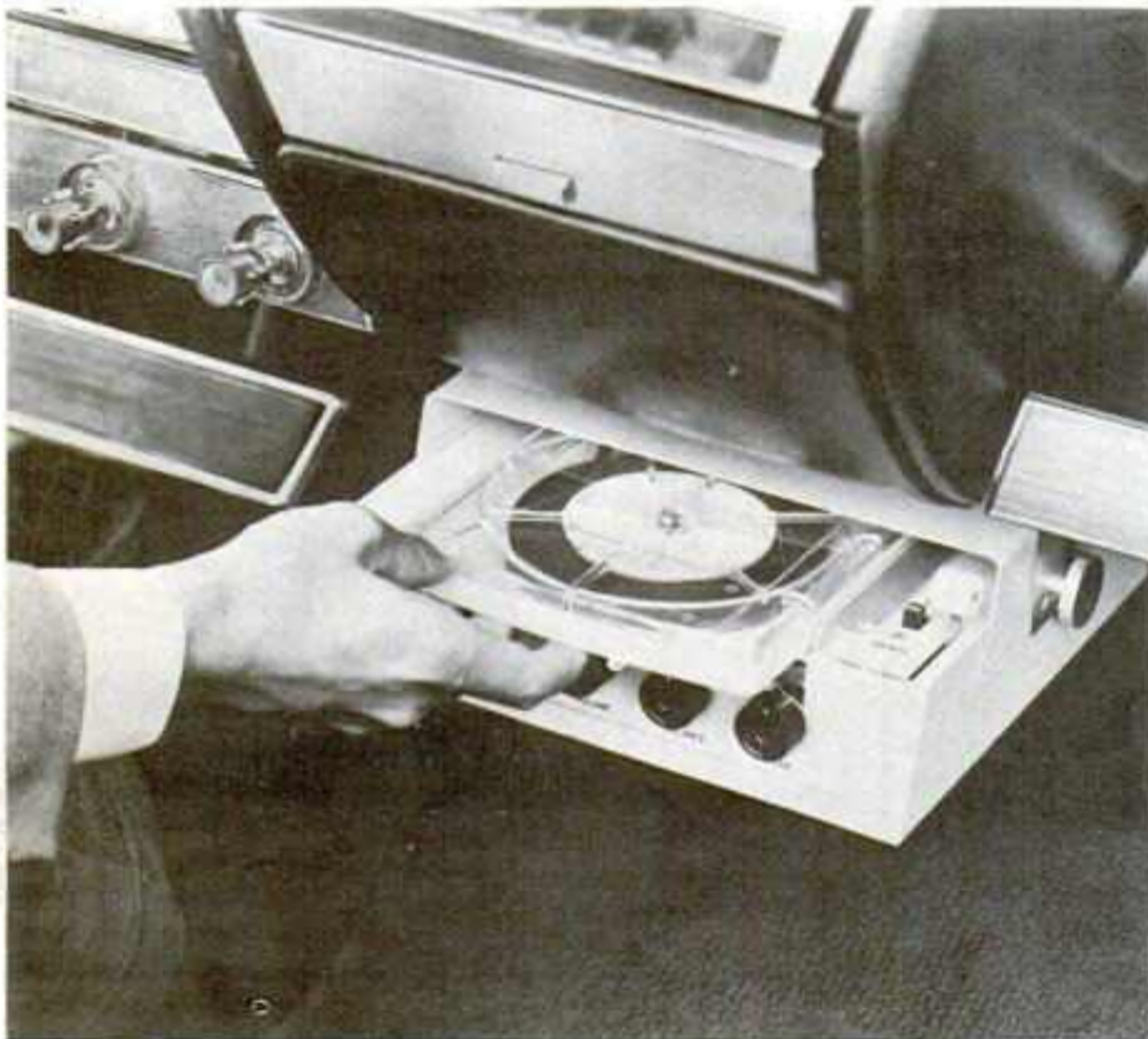
CLOSE-UP VIEW of Muntz Autostereo unit, with perpetual-play tape cartridge being slipped into playing position. Black knob in right foreground on top of deck activates tape head to permit listener to change music program on four-track tape from one double channel to the other. Multiple album cartridges are programmed to carry different and usually contrasting music on each of the double-channel bands.
