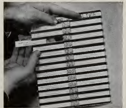
When changing a record, you remove only the slips for that record. You can change records one at a time without disturbing other program slips.
