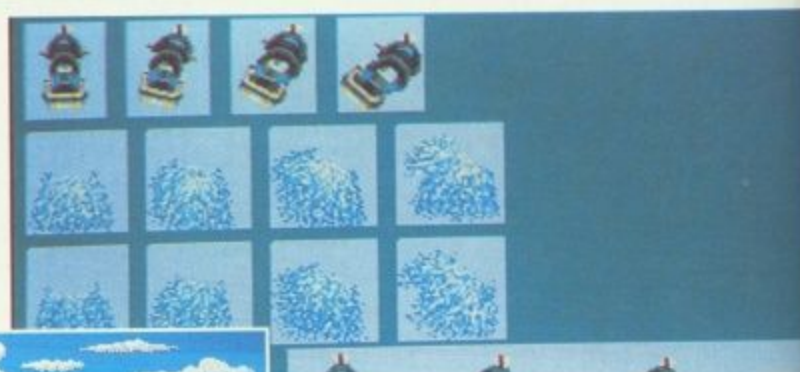
(Above) The trip across the Med takes place on the back of a jet ski. These sprite screens show some traditional memory saving tricks in action. Each object is only drawn turning to one side; if the opposite direction is needed the program flips the sprite before printing.
