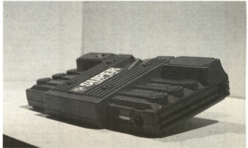
Sockets in the front of the Graphx accept PC Engine-style joypads while the expansion bus at the back could, were such things available, accept a disk drive and keyboard.
