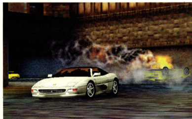
NFSIII's visual effects include reflective surfaces, particle systems, variable-density smoke, and projected lighting, with no hit on frame rate
