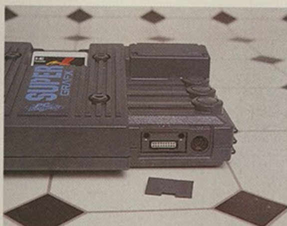
• Sockets at the front cater for the tiny but usable joypad and a mysterious 'S Expansion'
