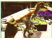
Once the whole thing has been baked in a special oven and the model removed from the mold, an airbrush artist paints it.
