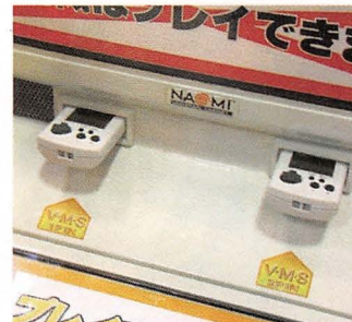
Sega's Naomi board (left). Naomi coin-ops will allow users to transfer data to and from Dreamcast consoles at home via the VMS units (right)
