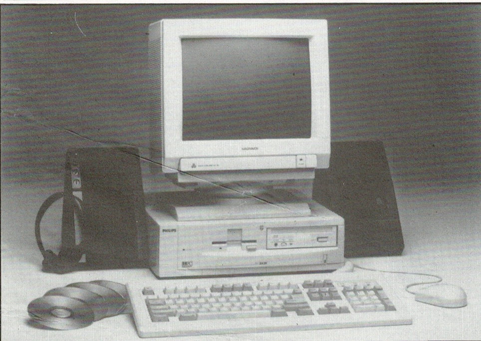
Above is Philips' contribution to the Multimedia PC (MPC) family. It bears the MPC logo — the trademark of the Multimedia PC Marketing Council, a gathering of various manufacturers pulled together by Microsoft which defined the standard. The 386sx 20MHz machine comes with an 80Mb hard drive and, of course, a built in CD ROM drive. It is currently on sale in the US and will arrive in the UK in the first half of 1992, although there are no details as yet of pricing and bundles.
