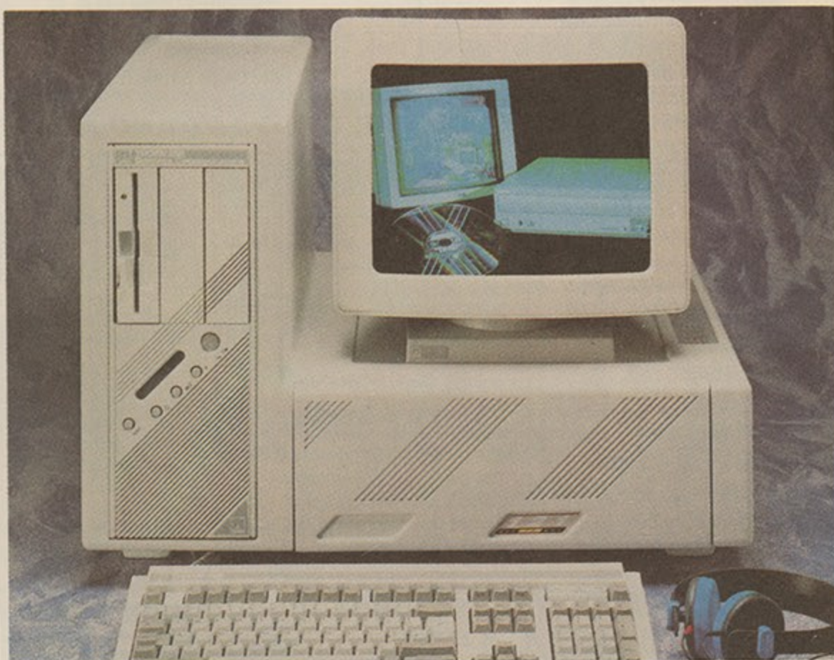
• Could this be the personal computer of the nineties? - 486 chip, six megs of RAM, built-in videodisc and CD quality sound
