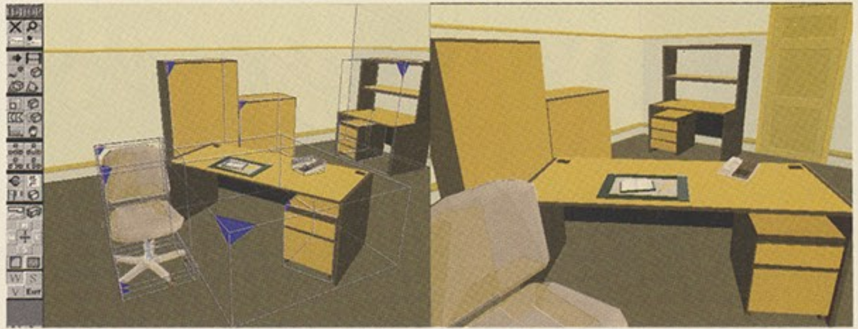
• Once objects are created in the shape editor they can then be placed into a virtual world model using the world editor. The chair in this picture can be moved and the desk drawers and cupboard doors opened
