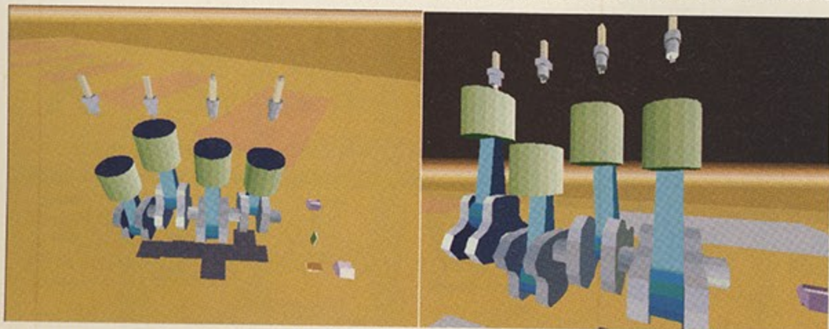
• Not just a graphical illustration of what's inside your car - the crankshaft, pistons and spark plugs in this image actually move to demonstrate how an engine's design works in practice
