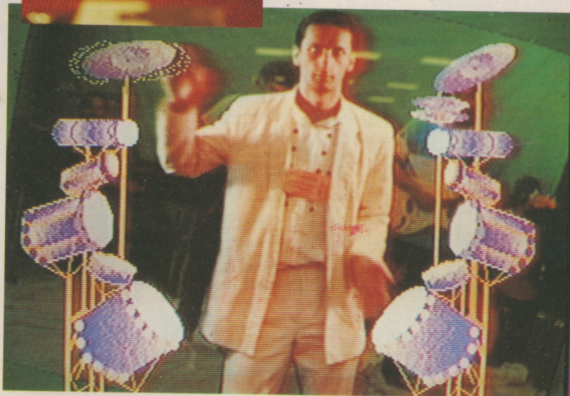
Top: Standing against a chromakey screen, a video camera records your image and sends it to a computer. Next, some computer graphics are added to the picture and then the software program – Mandella – takes over allowing you to inter-react with the combined image.
