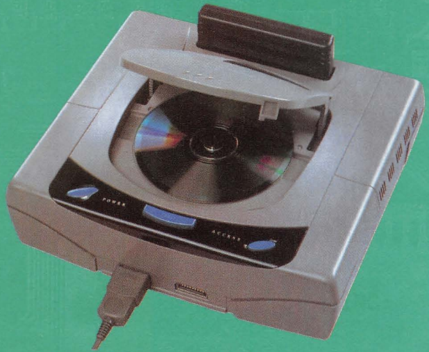
The Saturn's memory expansion slot enables future games to utilise extra ROM. So far, SNK is the only company to take advantage of this
