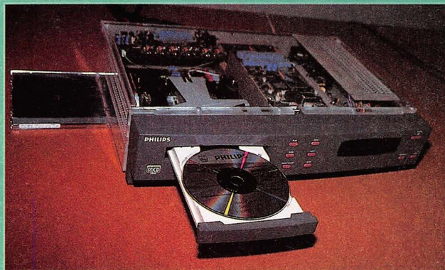
Digital Video Disc, while still seeking a final standard specification, offers a 4.7 gigabyte storage capacity on each disc. More FMV, then?
