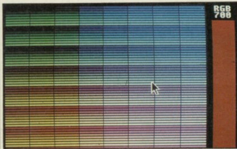
The rainbow-hued colour chart: one way of selecting a working palette - just click on the colour and the right-hand bar shows what you've got
