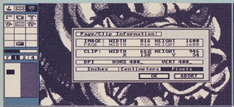
• The size of the clip area can be set more accurately from here, and the dots-per-inch information can be adjusted to suit the resolution of your printer.
