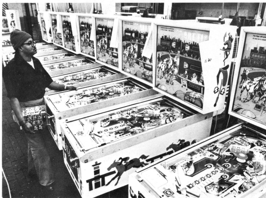
It takes several months to a year for a pinball game to develop from the first design sketches to actual production and distribution. Here, Hot Tip from Williams, passes through final inspection before delivery.
