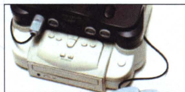
The Doctor 64 copying unit sits under the N64 and includes a CD-ROM drive
