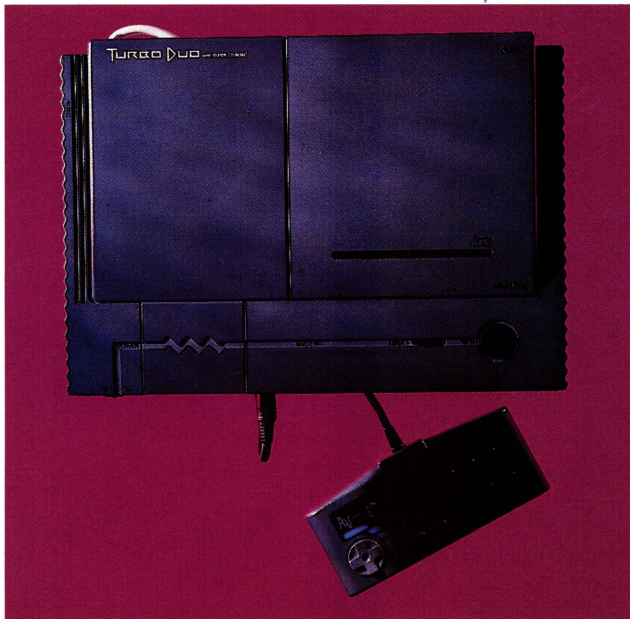
The American Turbo Duo – by far the most popular machine on import – also runs Japanese PC Engine CDs. Japanese HuCards need an adaptor
