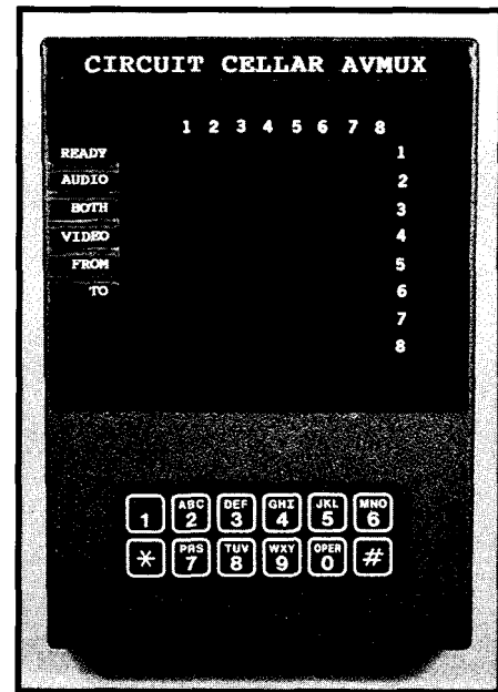
Photo 1--The 8x8 LED matrix makes for an easy-to-read panel when trying to discern which and what type of I/O connections have been made.
