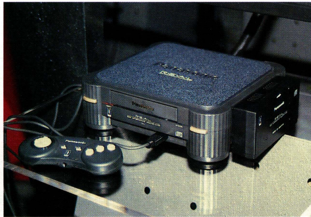
This device - the 3DO's MPEG cart - enables you to play White Book-compatible video CDs on your 3DO (see letter from Alan Nolan)
