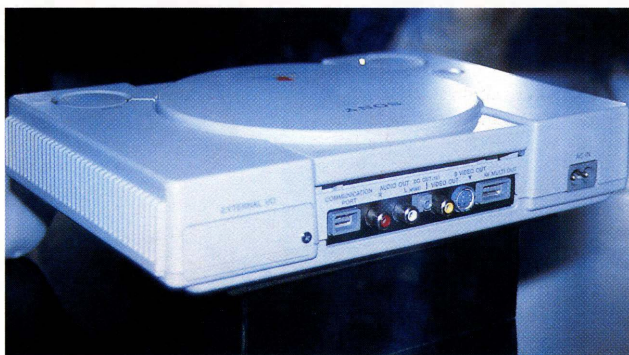
The PlayStation incorporates (from left) a comm port, stereo jacks, DC out (5V), composite video, S-Video, and an RGB AV multi-out
