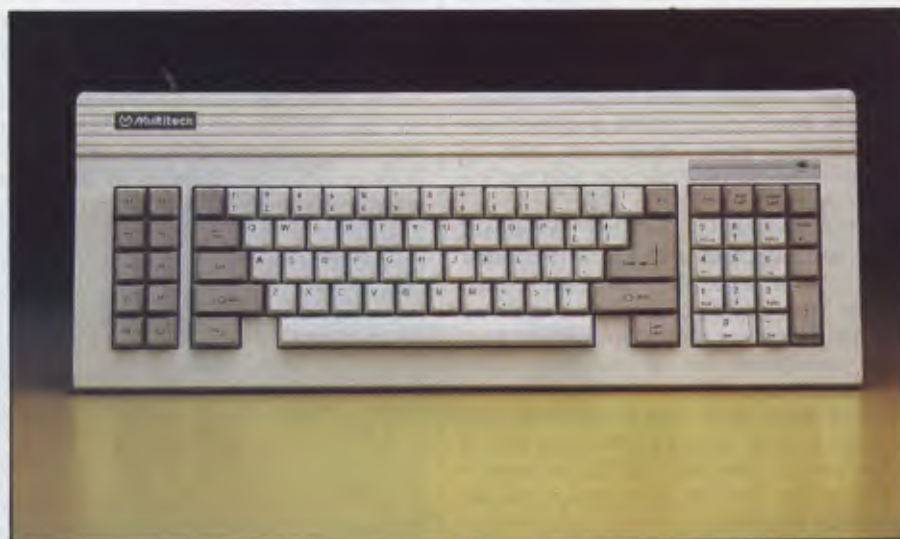
The 84 keys on the DSE/Multitech look straight off an IBM.
