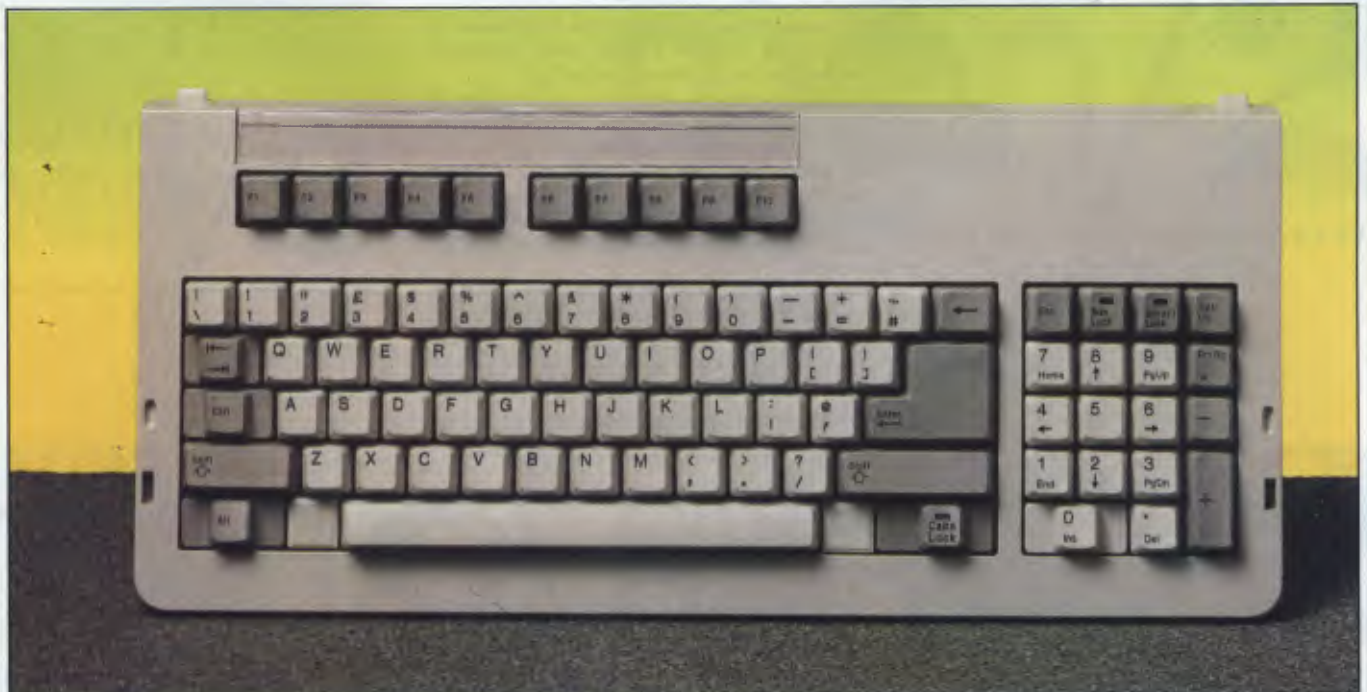
The 84-key keyboard is closer to the layout of the IBM PC/AT rather than the PC, but it still isn't truly compatible.
