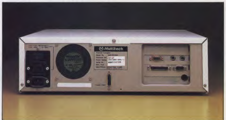
DSE provides more ports, but expansion potential is limited to one slot
