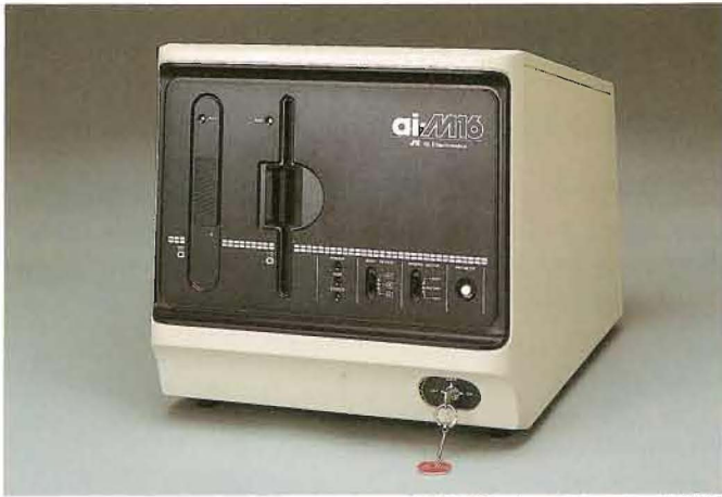
A powerful 16-bit microcomputer, ai-M16
