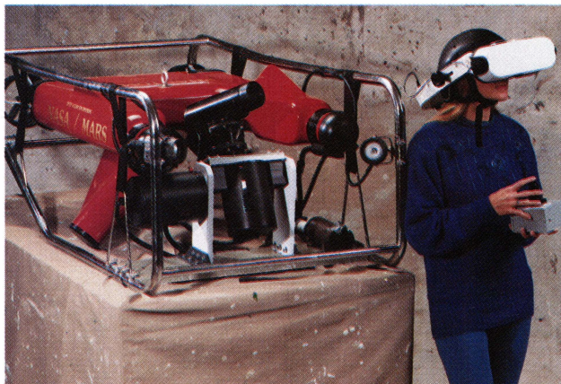
(Above) NASA scientists research the viability of telepresence using underwater ROVs linked to the controller via a stereo headset. (Left) A virtual ROV explores a Martian landscape generated by Sense8 Corporation's WorldToolKit
