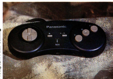
The FZ-JP1 joypad (left) is solidly constructed and very ergonomic. By unclipping the panel and plugging in another joypad (right), players are daisy-chained together
