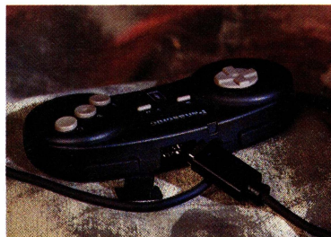
The FZ-JP1 joypad (left) is solidly constructed and very ergonomic. By unclipping the panel and plugging in another joypad (right), players are daisy-chained together
