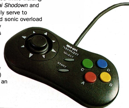
The new joypad (above) has a micro-switched directional control which works well. The rear of the machine features (from left to right) RGB SCART, S-Video, composite video and stereo jacks
