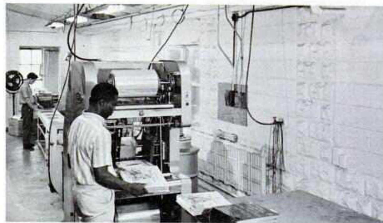
AT THE RECORDWAGON warehouse, only one operator is required to load disk packages into the Cryovac SA-1 machine, which then automatically overwraps, trims, seals and shrinks the film skin-tight at a rate of 1,800 units per hour.
