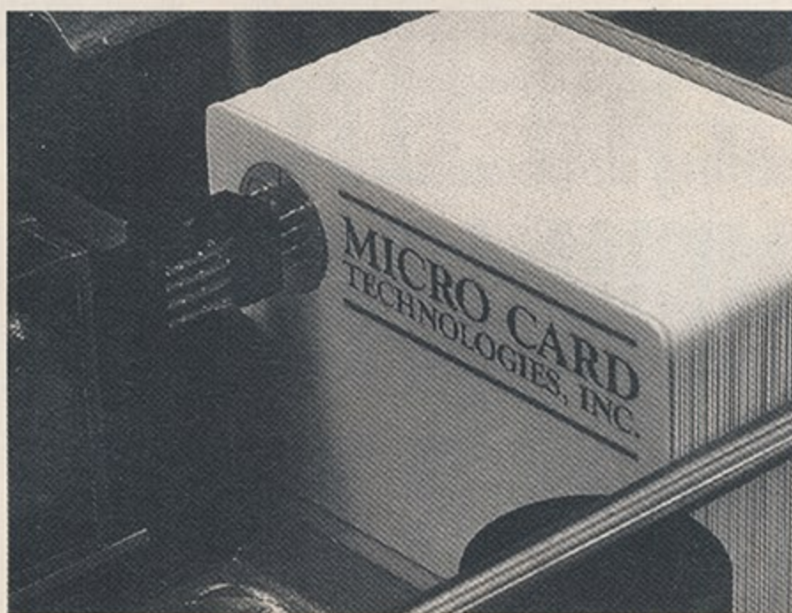
• Smart cards pouring off the production line: note the pins making contact with the card's chip.
