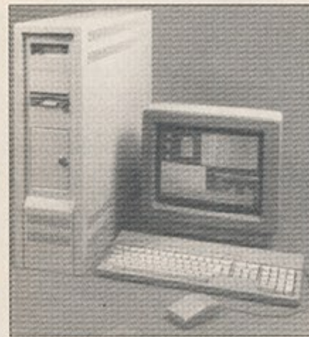
• Atari's ATW transputer-based computer, soon to be joined by a parallel processing model.
