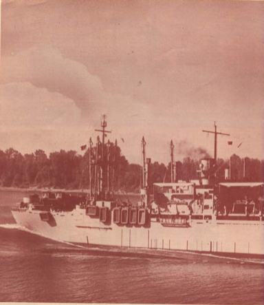
ATTACK TRANSPORT (VC2-S-AP5) The Attack Transports, or AP-5s, are armed troop transports built on Victory ship hulls. As the war against Japan began to move faster than originally scheduled, they became urgently needed. Contracts were awarded to the four fastest yards in the nation, Oregon,
