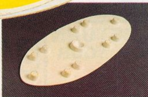
Your bespoke plastic surfboard featured special underside protrusions to punish those rubber keys.
