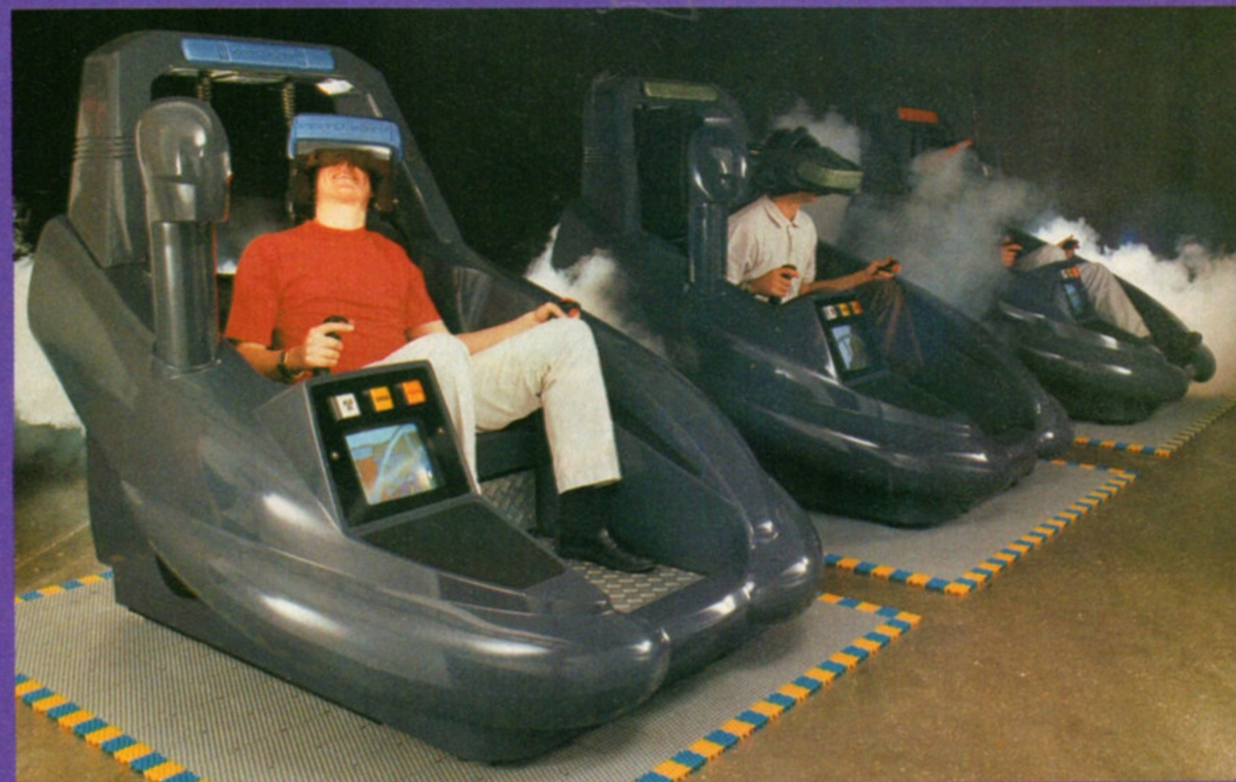
Virtuality 1000 SD, a high quality, sit-down console which enables the operator to drive the 'vehicle' in a virtual world
