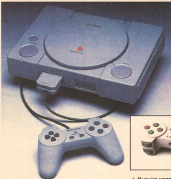
▲ If you're wondering why the joystick plug is so thick, it's because the slot above the joystick fits a RAM card for saving games etc.
