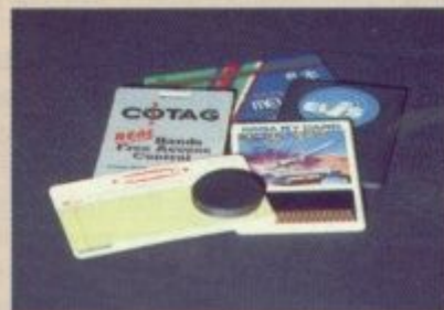
The smart cards. From bottom left moving clockwise: LaserCard, COTAG, MELCARD, ELIS and Sega My Card. The large black disc in the foreground is the other version of the ELIS card.
