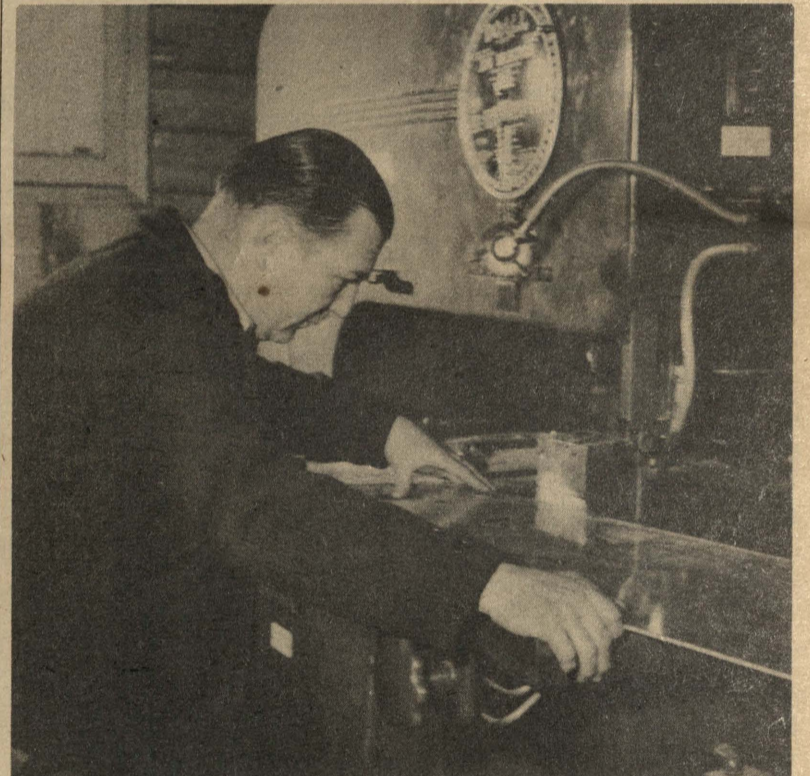
Cutting of small aluminum parts for pontoons on the Doall saws began last week. The highly efficient power saws, such as the one shown above being demonstrated by Leo Redding, Plate shop foreman, welds, anneals and adjusts its own saw blade mechanically, completing the process in less than two minutes. Much adjusting of the machine is done by use of a "job selector" dial which can be set for file type, cutting velocity, saw temper, saw set, power feed and saw pitch.
