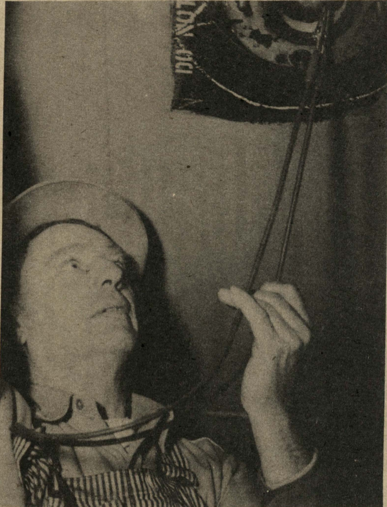
Running a weak electric current through fine wires glued under deck plates is the chore of P. B. Wright, shown above. His test wires are connected to the calibrating instrument being read by other crew members to determine weld stress in deck plates. Wright is a former OSC plant protection engineer.
