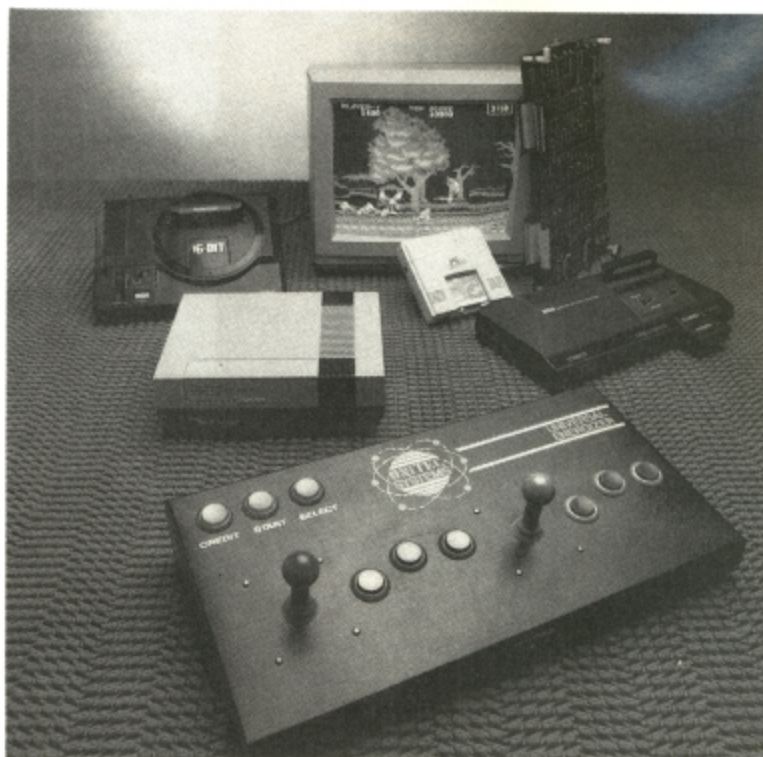
The Universal Energizer from Unitec lets you control consoles, computers and coin-ops. A jamma interface at the back of the machine means arcade boards can be plugged in and played on your TV or monitor.
