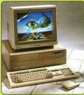
For the more serious or professional applications user, Commodore have a selection of systems based around the expandable Amiga 2000, at prices from £1295+VAT. The A2000 features a full 1Mb RAM (expandable to 9Mb), 9 system expansion slots, plus IBM compatibility with the use of PC-XT or PC-AT bridgeboards. Complete and return the coupon, putting a tick in the A2000 box, for details of A2000 computer systems.
