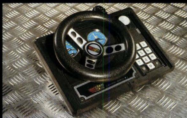
The ColecoVision's 14-button controller was lauded for its flexibility – Atari's VCS equivalent had one solitary fire button. The Turbo module for the game of the same name (right)
