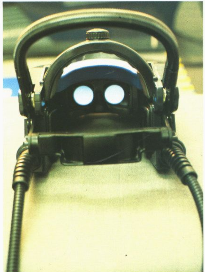
The goggles use twin displays of remarkable clarity to generate stereoscopic views - and you get stereo sound as well n"
