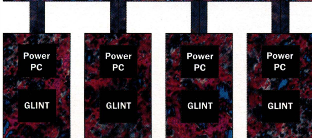
The parallel architecture of Tao's arcade system features four PowerPC chips and four GLINT chips – seriously powerful kit
