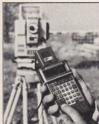
Automatically records distances and angles.
