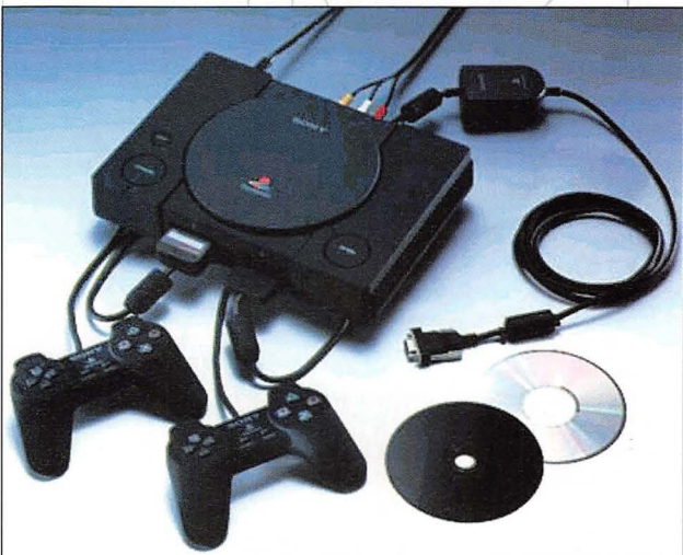
The Yaroze development kit, complete with system and libraries discs and computer interface lead - but not territorial lock-out chip
