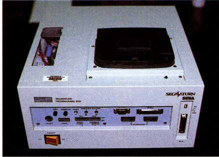
Previously, the Saturn development system included a P-Box, or programmer box (left), instead of a production Saturn. In the new system the P-Box has been replaced by SOA's CartDev box, which sits below the Saturn, and a cartridge which interfaces with the PC or workstation. Sega's 'official' development set-up (right) includes an SGI Indy, Softimage, CartDev, SNASM2, and AM2's SGL
