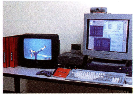
Previously, the Saturn development system included a P-Box, or programmer box (left), instead of a production Saturn. In the new system the P-Box has been replaced by SOA's CartDev box, which sits below the Saturn, and a cartridge which interfaces with the PC or workstation. Sega's 'official' development set-up (right) includes an SGI Indy, Softimage, CartDev, SNASM2, and AM2's SGL
