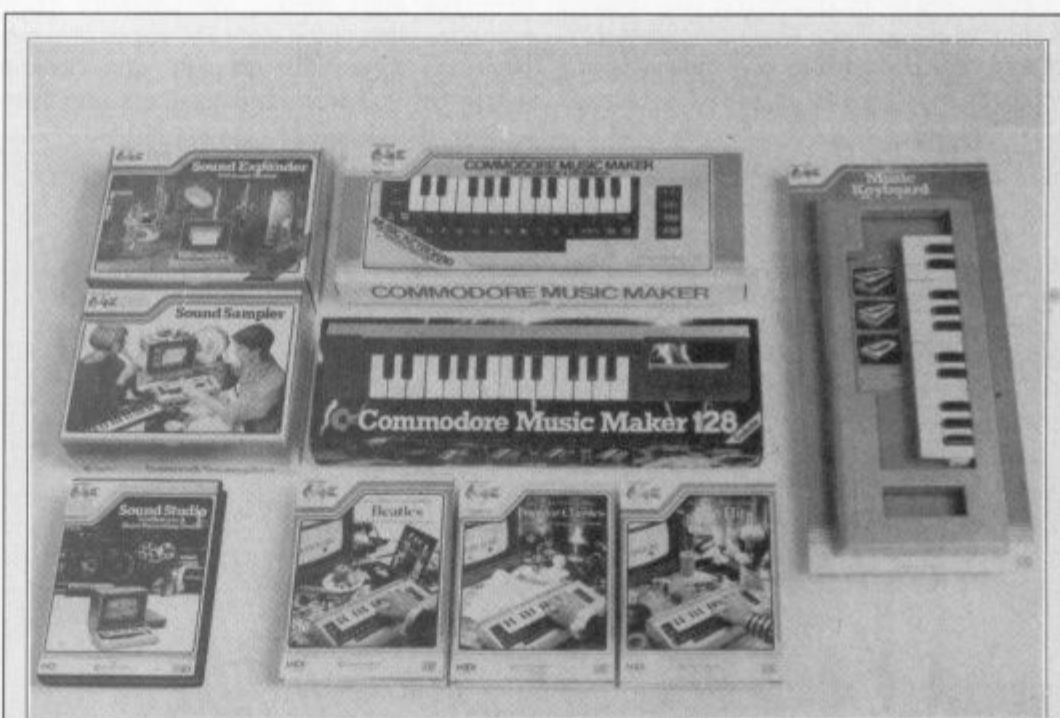
If you want to 'sing something simple', you could try the Commodore Music Maker, which gives you a mini plastic keyboard to fit over the top of your 64, together with software that enables you to make easy use of the computer's sound chip. There are a number of add-on packages and you can also get a system designed to fit over the Commodore 128 (which the 64 version won't work with, due to the different design of the keyboard). Fun for the kids, but don't expect much in the way of sophistication unless you go for the Sound Expander (see elsewhere). Prices vary - shop around for best deal.
