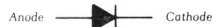
Fig. 1-1B. The standard symbol for a semiconductor diode. The arrow indicates the direction of current flow (the standard of this text) while the labels are consistent with the electron flow convention.
