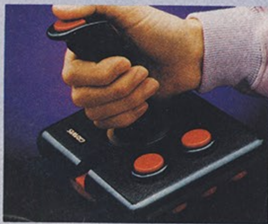
• The Advanced Gravis joystick, featuring unique tension adjuster
