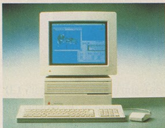
• The top of the range, the Mac IIci, a 68030-based powerhouse with 4Mb of RAM and an 80Mb hard disk
