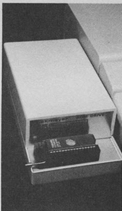
• Lakmeyer's new EPROM programmer can turn chips into a read-only second drive
