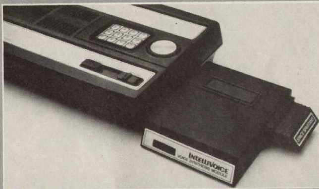
The Intellivoice voice synthesis module attaches to Intellivision producing male and female narration.
