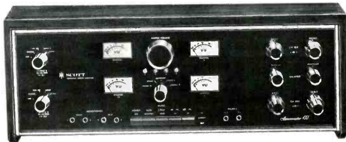
4-CHANNEL stereo amplifier. H. H. Scott, Inc. claims that this is the first commercial amplifier specifically designed for 4-channel stereo. Called Model 499, the unit will play the new 4-channel pre-recorded tapes and is compatible with existing 2-channel stereo systems. List price is $599.95.
