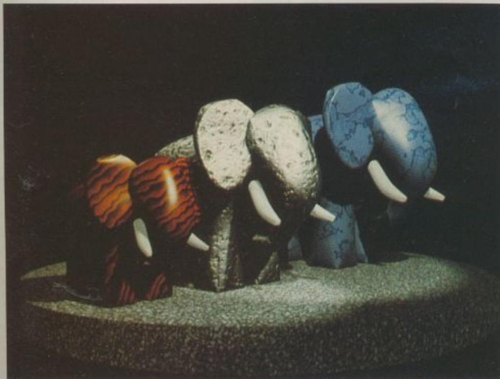
The Renderman graphics language includes special commands that can mimic real world textures. In this image, you can see the use of the shading commands WOOD0 , DENTED0 , BLUE_MARBLE0 , and GRANITE0 .
