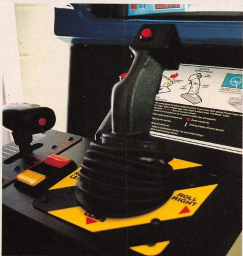
Top: Silent Service II - out soon on PC, and a candidate for coin-op conversion? Bottom: Controls on the coin-op are simple and easy to use. Joystick houses fire button, target lock-on, and missile fire switch; thrust control on the left also houses afterburner. Decoy release button is on fascia. Joystick control is very sensitive - this is no sluggish 16-bit flight sim, this is FAST
