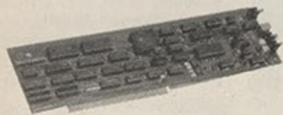
• The AD2105 from SunRize. It offers 12-bit sampling and SMPTE time codes.
