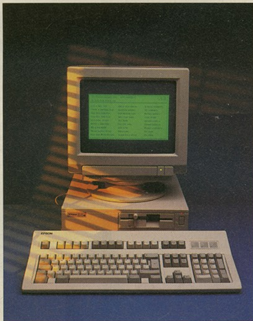
• The TriGem 88e bundle includes a Philips Professional 7BM713 monochrome monitor and an Epson enhanced/AT style keyboard with 12 function keys.
